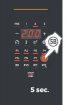
By choosing a different position, for example P8, program P7 will keep its original settings (i.e. the temperature at 180°C), while program P8 will have the same parameters as P7 except the temperature will be 200°C.
