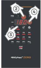
In this example, program P7 needs to be modified, increasing the temperature of STEP2 from 180° to 200°C.
