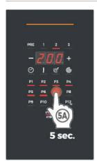
By pressing the P7 button again, the program is overwritten i.e. changed permanently. This means that, from now on, the P7 program will have a temperature of 200°C instead of 180°C.
